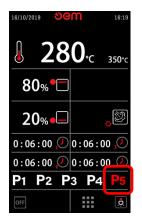
After modifying any parameter (set temperature, timer, etc.), the indicator of the program in use (for example P5) will begin to flash. This indicates that a parameter within the cooking program has been changed but has not been saved.
