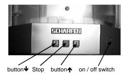
Never move the knife set upwards in case there is still cheese in the machine. This can cause damages at the machine.
