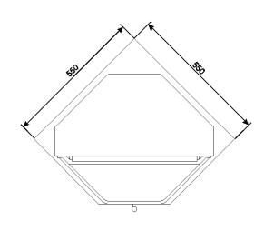
overall dimensions 550 x 550 x 550 mm counter space required 400 x 350 mm
