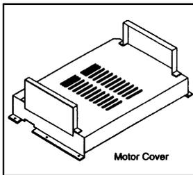
12. Attach Motor Cover as shown with bolts provided.
