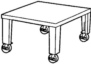
1. The stand is a 40" (1016 mm) x 49" (1245 mm) rectangle. Set it in place with a 40" side facing out. This will be the front of the oven. Using a carpenter's level, level all four (4) sides of the stand. To raise or lower the stand use the leg adjusters. Ovens on casters require a level floor. NOTE: The oven top is packed with oven stand. Remove top from stand before assembly.
