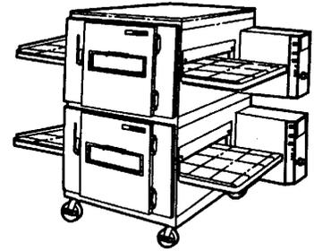
3. If you purchased a double stack oven, place the second oven on top of the first one. Be sure that it sets on squarely and is fully seated. The control panel goes on the right rear. Now install oven top.
