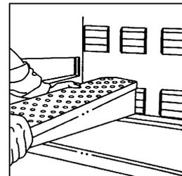
9. Insert assembled finger through door opening starting with lower left. NOTE: The customer MUST tell you what position to place the assembled finger in, for their application.
