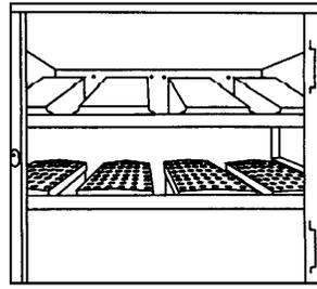
10. Install finger in the oven by sliding it over the plenum flange and setting the front bracket. **BE SURE THAT THE FINGER SETS SQUARELY OVER THE PLENUM FLANGES AND THE HOLES POINT IN THE PROPER DIRECTION. Top fingers point down, bottom fingers point up.**
