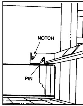
5. Rotate the finger brackets until the notches in the brackets sit on the retaining pins.
