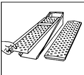
7. Insert columnating plate so the step goes under the lip of the finger housing and the plate lies flush with the housing side edge.
