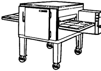
2. Remove the oven from the dolly and set it on the stand. The control panel should be on the right rear as you face the oven. Be sure that the oven sets squarely on the stand and is fully seated. For a single oven, install top. For double, see step 3.
