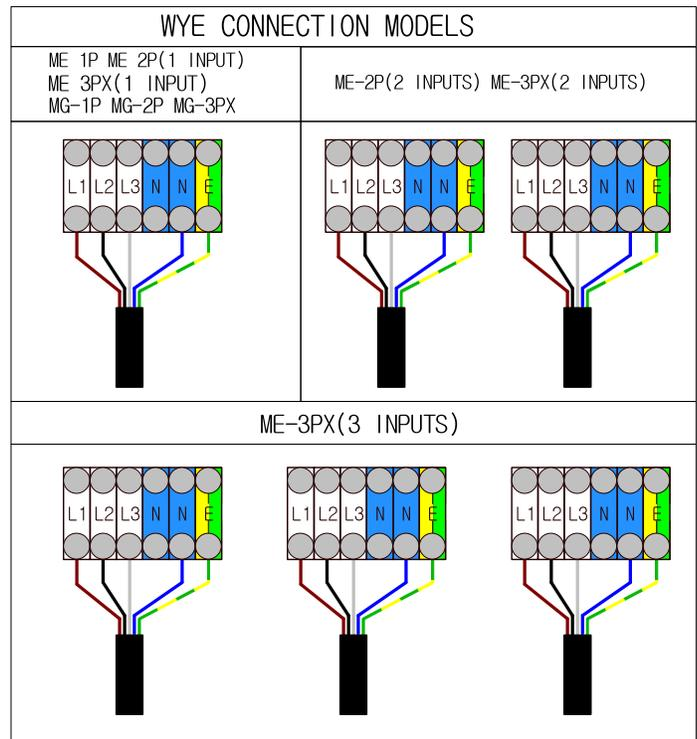
**Power Interlock Terminal Block Diagram**
