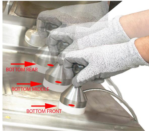
**Placing Pyrometer to the Top Platen.**
