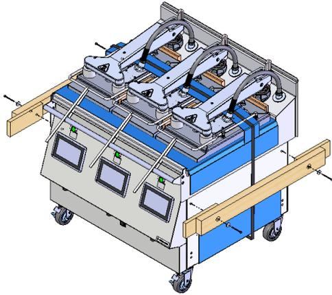
8. Remove and discard the wood blocks attached to the sides of the grill using a Phillips screwdriver (PH2)/square drive (S2).
