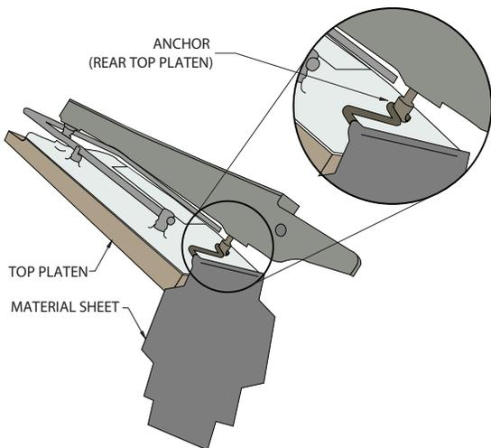
4. Gently pull the release material sheet towards the front platen and then wrap the sheet around the front of platen and over the U bar, while holding the front end sheet, place the locking clip over the sheet and press into the rod.
