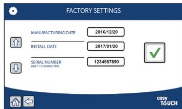
6. Type the date of installation and then press the check-mark to save.
