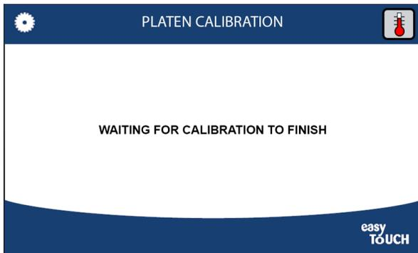
NOTE: as soon as the grill has completed the preheat, the computer will take control of calibration. During this process the top platen will move up and down. Do not interrupt the calibration process.
