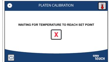
**Tip:** Pressing the thermometer icon (top right corner) temperature status will pop-up and display the actual temperature of the grill.
