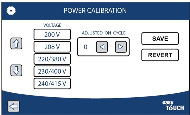
4. Using the up or Down arrows select the appropriate voltage of the grill. Each controller is independent, select the voltage calibration on each controller.
