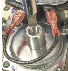
b. remove the sealing cap on the gas valve regulator
