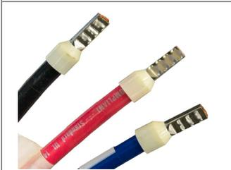
Note: ensure all wires has terminal pin installed and crimped to each wire end.
