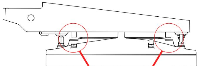
Sensors (Proximity & sensor target) must be kept clear & clean at all times.
