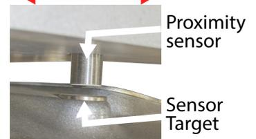
Proximity sensor is used to detect the position of the platen using the sensor target attached to the platen cowl, conduct "visual inspection".
