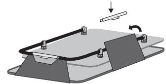
6. Check alignment and tightness of release material against the upper platen. Make adjustment if necessary.
