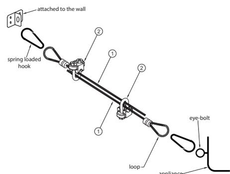
6. Attach one of the spring-loaded hooks to the bracket on the wall and the other end to the eye-bolt (grill). adjust the proper distance of the cable (1) and tighten both clamps (2) to secure the cables.
