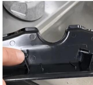
3. Grasp the Splash Shield using the finger handle on the front.
