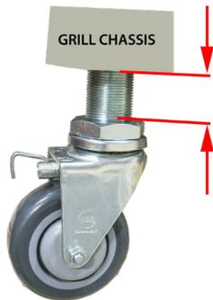
Beware of the red mark on the caster stem. The red mark indicates the maximum adjustment position and must not be visible after adjustment, before the jam nut is tightened in place.
