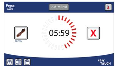
3. An audible warning sounds prior to the end of the cook cycle. When the cook cycle has finished, the platen lifts. Press the check mark or the Green button to clear the message.
