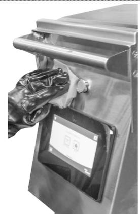
27. Wipe grill side surfaces with a clean, sanitizer-soaked grill cloth. Remember to clean always in the direction of the grain. Do not remove panel by any circumstance, if grease migrate inside the grill call service technician for support.
