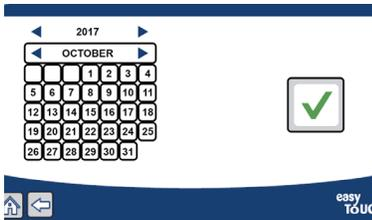
7. Verify the installation date and the serial number then press the check-mark to save.
