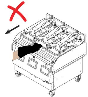
DO NOT MOVE GRILL USING THE MATERIAL SHEET U-BAR.
