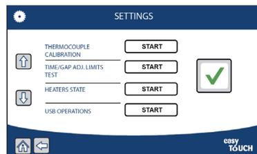
4. TIME & GAP ADJUSTMENTS screen: set to zero to prevent users from adjusting the cook cycle.
