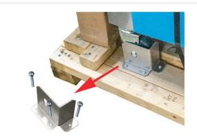
6. Remove and discard the metal bracket attached on the rear casters by using a Phillips screwdriver (PH2)/square drive (S2).
