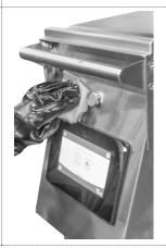
27. Wipe grill side surfaces with a clean, sanitizersoaked grill cloth. Remember to clean always in the direction fo the grain. Do not remove panel by any circunstance, if grease migrate inside the grill call service technician for support.
