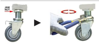
11. Move the Jam Nut up to the top, do not tighten. If the grill is uneven gently place a pump pliers in the lower part of the threaded stem and turn it clockwise to increase or counterclockwise to decrease the height of the grill to level the grill according to the levelling tool reading.
