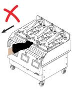
DO NOT MOVE GRILL USING THE MATERIAL SHEET U-BAR.
