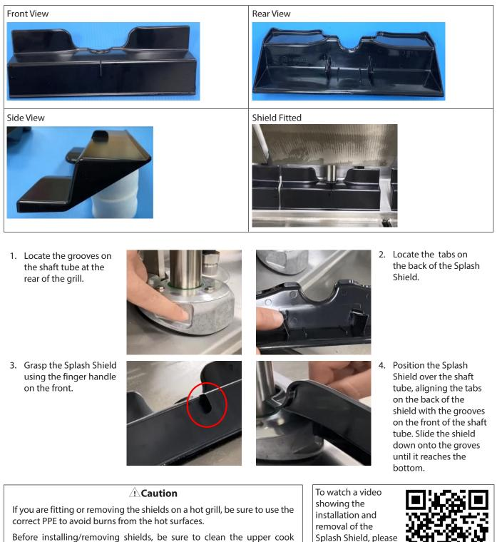
surface to avoid exposure to hot dripping grease. Do not use damaged shields, discard them and order replacements by Splash Shield, please scan the QR code. Then go to Crew, then Videos.
