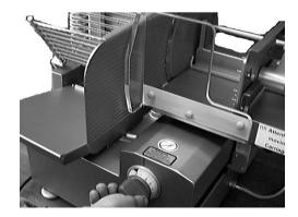
there is flashing on the display the value for the thickness of slices, you have to adjust with the thickness knob a value >0.4. Then start again.
