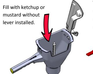
With a clean and empty dispenser add ketchup or mustard BEFORE installing lever. If dispenser has run out of sauce during use it can be refilled without removing lever.
