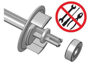
Install and replace piston rings and springs by hand, do not use tools or sharp objects. Mustard piston ring shown.
