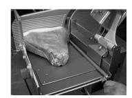
Move the carriage by hand forward and backward by using the handle in front of the carriage. It is necessary that the carriage is always pushed to the utmost end position, because only then the stacking procedure will be triggered off.
