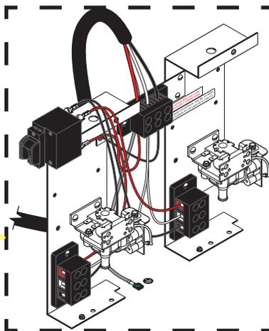
**Note:** Power cord must be connected to center terminal block on all Twins unless otherwise noted.
