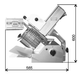
overall dimensions 670 x 565 x 600 mm counter space required 580 x 390 mm max. cutting size app. 210 x 175 mm thickness of slices (infinitely variable) 0 – 10 mm Manufacturer: Hermann Scharfen GmbH & Co. Maschinenfabrik KG Ruhrstr. 76-76a, D - 58452 Witten, Tel. 02302/282770
