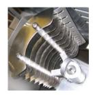
Now you can mount the **stacking comb** onto the second shaft. Please see to it that the small bolt of the spiked slice catcher is situated correctly between the shaft and the plate springs. Only push the stacking comb, do not turn it as otherwise the plate springs can break.
