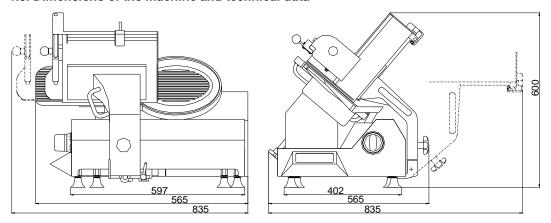
overall dimensions 728 x 565 x 600 mm counter space required 597 x 402 mm max. cutting size (blade 300 mm) app. 305 x 210 mm max. cutting size (blade 330 mm) app. 305 x 225 mm thickness of slices 0 - 25 mm (infinitely variable) Manufacturer: Hermann Scharfen GmbH & Co. Maschinenfabrik KG
