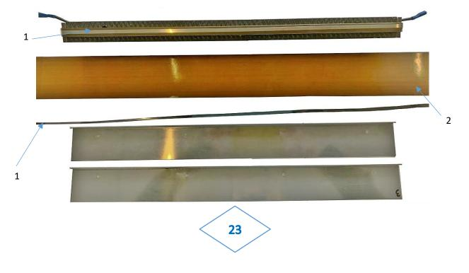
• Replace welding diaphragm when needed. (if broken or if it loses pressure during the sealing).
