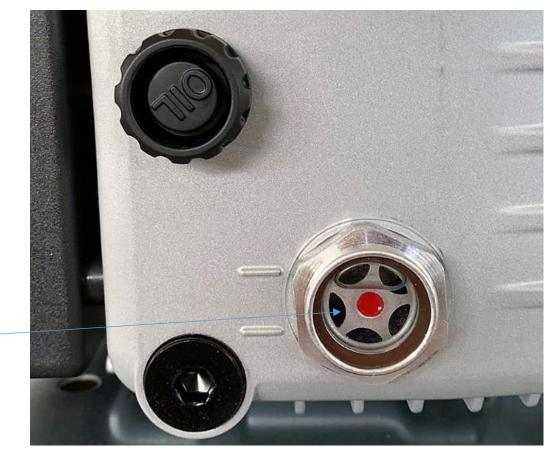
Before starting, check oil level through the small window on the motor (Picture 1). To reach the window, unscrew the 4 screws which block the back of the carter and (for (for models with oil pump) turn the carter frontward at 90°.
