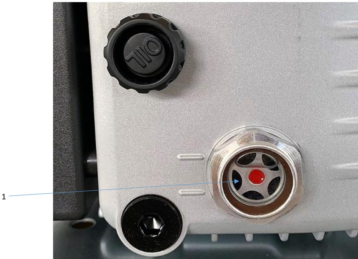
Before starting, check oil level through the small window on the motor (Picture 1). To reach the window, unscrew the 4 screws which block the back of the carter and (for (for models with oil pump) turn the carter frontward at 90°.
