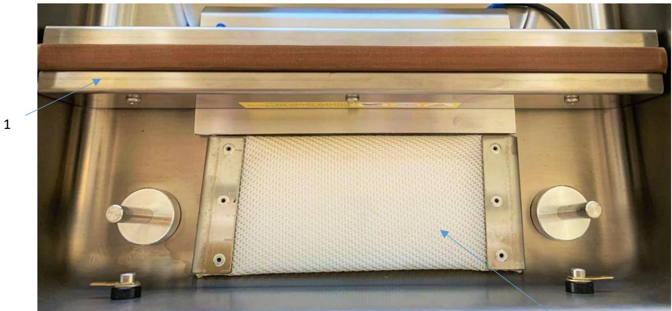
Picture A: Sealing bar with diaphragm
