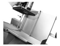
Take off the blade guard and lubricate the threaded bushing, the adapter, and the fixing screw of the blade guard (we recommend Autol Top 2000, which is used in our factory)
