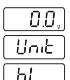
⇒ Keep pressed in the weighing mode until "Unit" is displayed.
