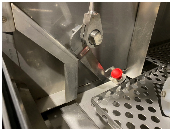
Fig. 49 The upper door is loose
