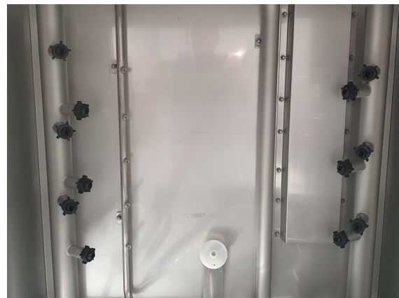
Fig. 74 Mounting new nozzles. Do not overtighten!
