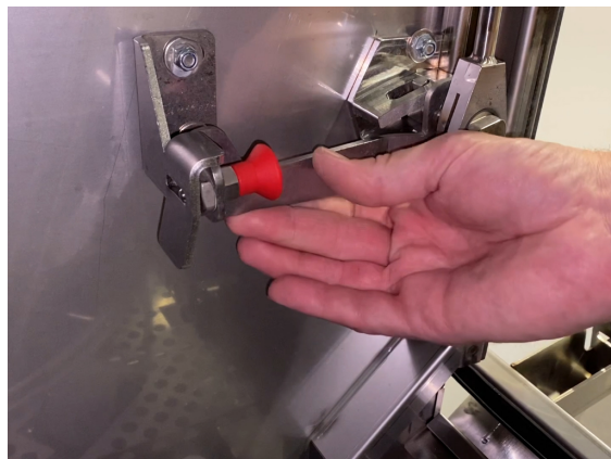
Fig. 55 Close up — secure the arm properly
