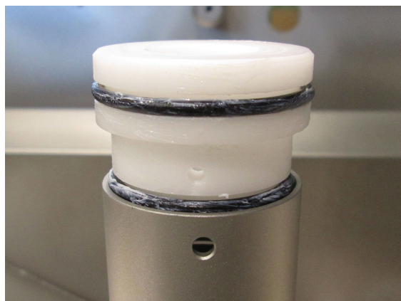
Fig. 79 Replace the O-rings and apply grease.
