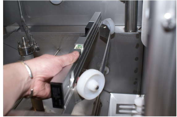
Fig. 63 Levelling the machine, side.
