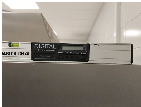
Fig. 4 Leveling right side, do the same on the left side.
