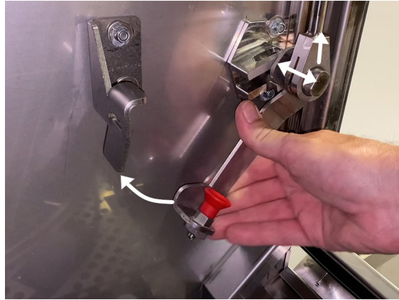
Fig. 53 Securing the locking arm
