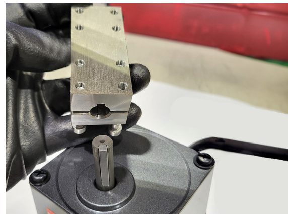
Fig. 59 Mount the coupling onto the new drive motor
