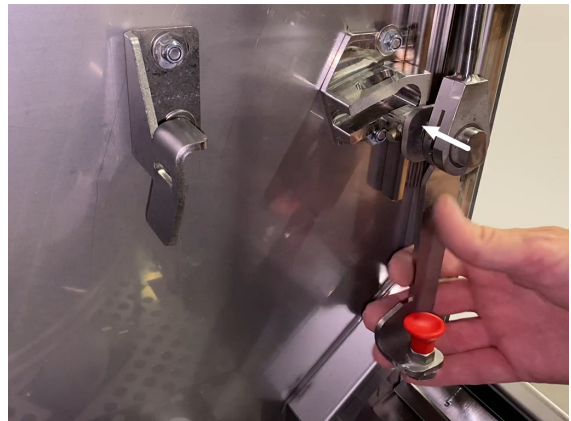
Fig. 52 Insert the shaft in the seat of the housing
