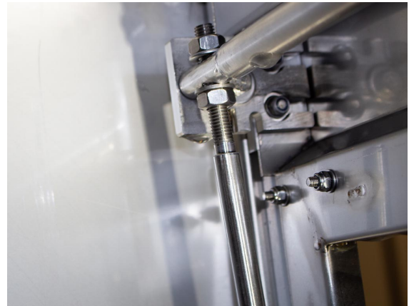
Fig. 64 Rod with lock nut for adjustment.
