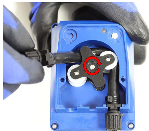
Fig. 69 Turn the roller according to the arrow (clockwise)
