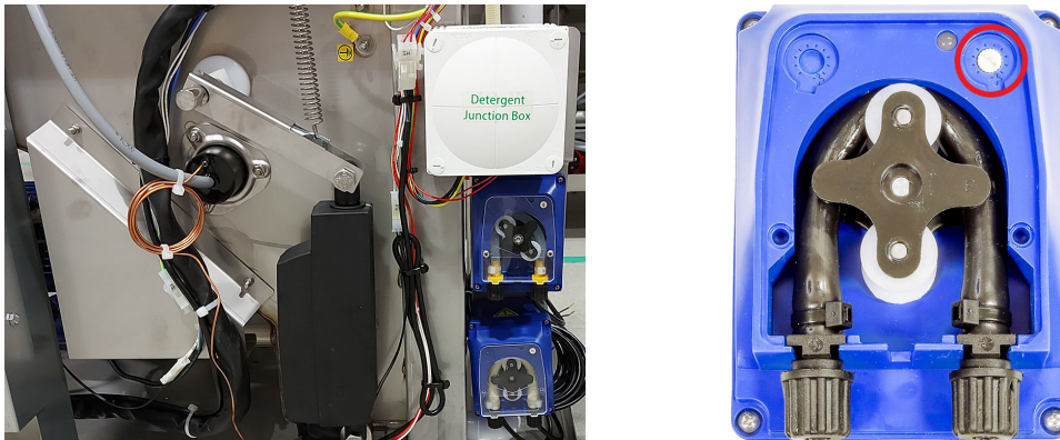
Fig. 15 Dosing pumps - Adjusting the trimmer
