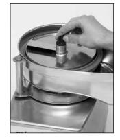
Next fit the appropriate slicing disc and screw the slicer on the motor shaft with the butterfly nut.
