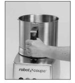
3) Engage the blade on the motor shaft and lower it right to the bottom of the bowl.
