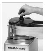
3) Slot the grey plastic ejector disc onto the motor shaft and check that it is properly positioned at the bottom of the bowl.
