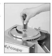
• Position the automatic hopper on the motor base. The fastening hook is now facing you on your right.
