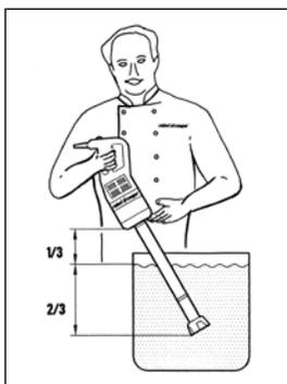
The power mixer can equally be rested against the rim of the container, but must be tilted, and the bell must not touch the bottom of the container.
