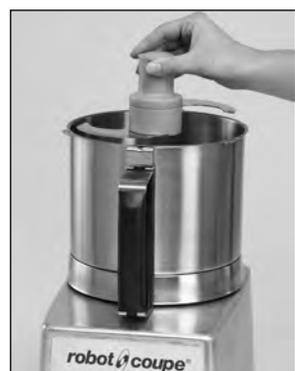
3) Engage the blade on the motor shaft and lower it right to the bottom of the bowl.
