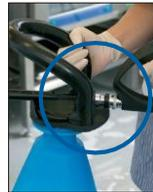
6. The water gun (item no. 53105A1 or 40801A3) is connected to the nipple on the injector.
