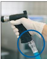
7. The hose with 1/2" quick coupling (item no. 5350SA3) is connected to nipple on the water gun.
