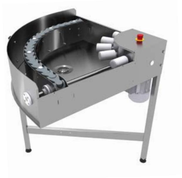
Motor-powered turn track made entirely from stainless steel. Frame made from non-corrosive, 30x30 mm square tubing with adjustable feet. Suitable for all 50x50 cm washing baskets. The design means that the baskets are loaded using a plastic drive chain. Equipped with an emergency stop.
