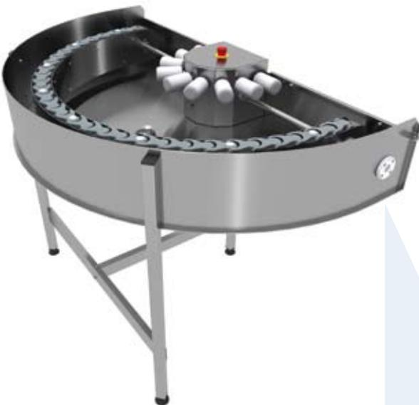
Motor-powered turn track made entirely from stainless steel. Frame made from non-corrosive, 30x30 mm square tubing with adjustable feet. Suitable for all 50x50 cm washing baskets. The design means that the baskets are loaded using a plastic drive chain. Equipped with an emergency stop.
