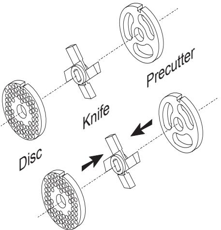
The knife must be replaced or grinded when the wearing surface on the side of the knife is more than **1 mm**. If this is not done, the mixer can be damaged, as the friction in the meat mincer is increased when the knife is worn.
