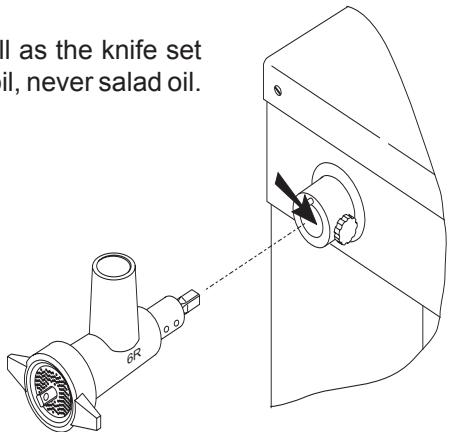
If the feed screw is stuck, when the meat mincer is to be disassembled, it can be pulled out by inserting a hook or a similar tool in the hole of the feed screw shaft.
