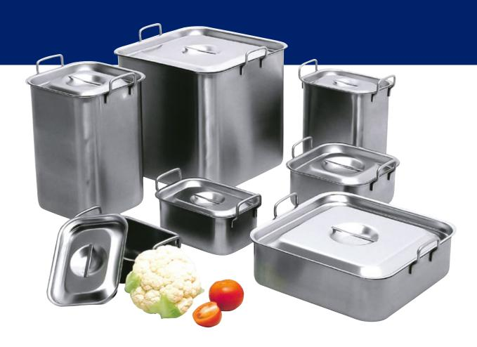
ABC containers are manufactured in high quality 18/8 stainless steel, electrolytically polished to a finish that satisfies the highest hygienic demands. They fulfil the European Norm for materials used in connection with food processing, EN 631. Extensive service life is guaranteed through the use of 0.8-1 mm thick steel.
